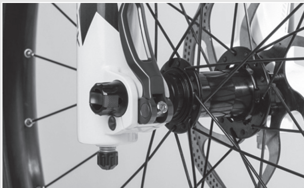
Figure 35: Perfect position for the clamping lever
