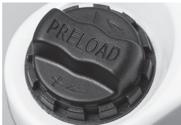
Figure 58: Negative deflection setting wheel on the suspension fork crown
