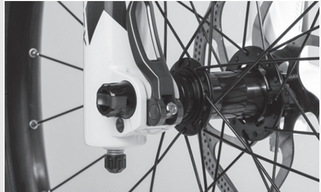
Figure 84: Adjusting the quick release clamping force
