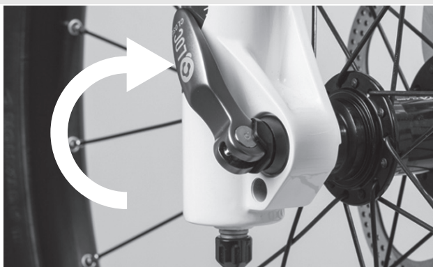
Figure 40: Closing the quick release
