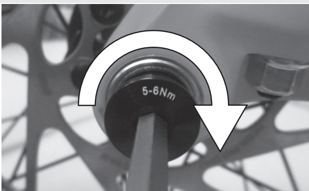
Figure 28: Tightening the securing screw
