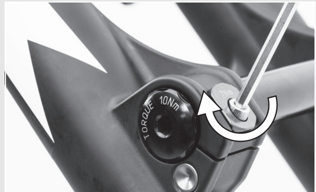
Figure 30: Tightening the axle
