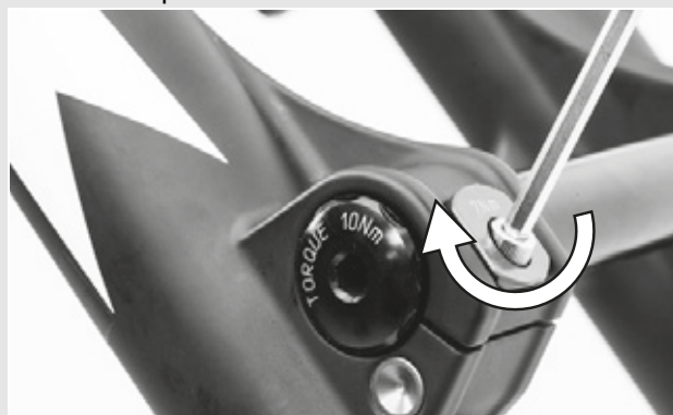
Figure 29: Tightening the securing clip
