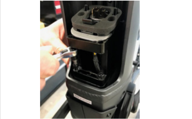
Figure 19: Removing the 4 mm hexagon screws
