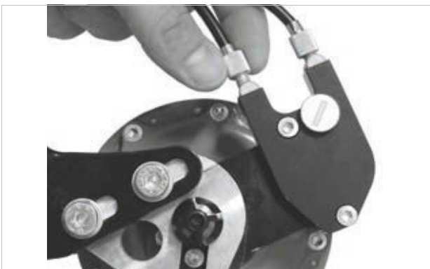
Figure 255: The tension adjuster on ROHLOFF hub versions with external switch control is located on the cable box positioned on the left-hand side
