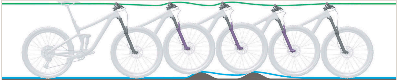
Figure 270: Suspension fork rebounding too slowly
