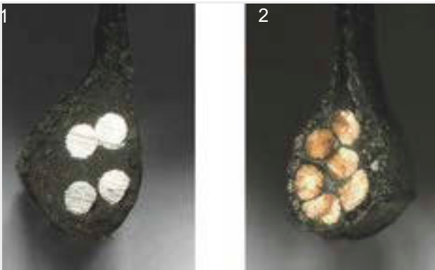
Figure 32: Steel bead core (1) and Kevlar bead core (2)
