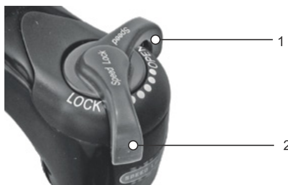
Figure 116: Suntour compression adjuster in open (1) and closed (2) position
