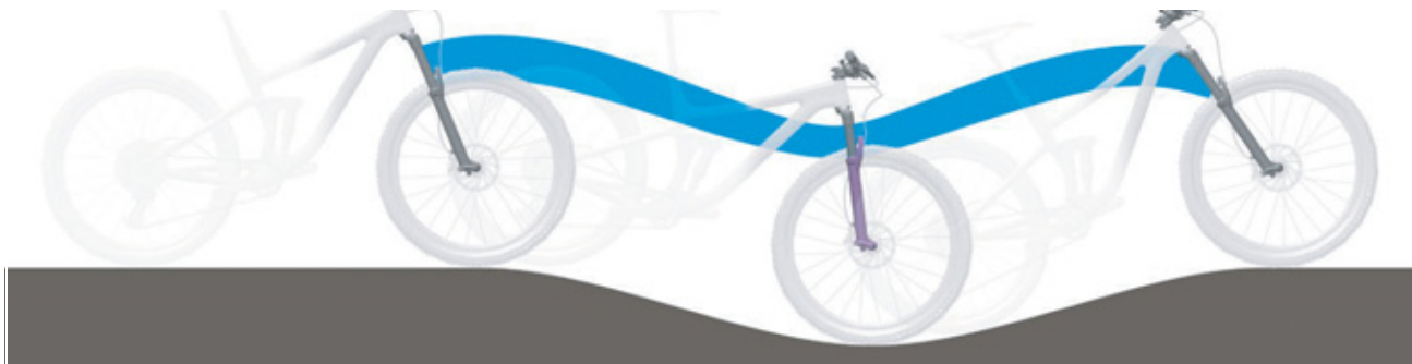
Figure 6: Optimum fork riding performance on hilly terrain
