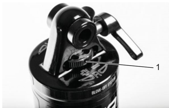
Figure 88: Suntour rebound adjuster wheel (1) on the rear frame damper
