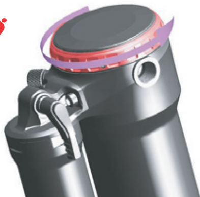
Figure 139: Turning rebound damper towards hare symbol
