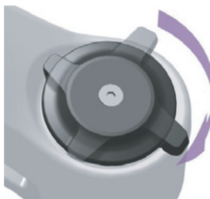
Figure 117: Changing compression adjuster to a harder setting
