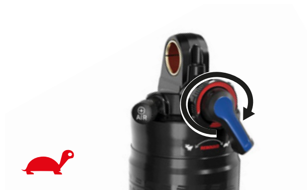
Figure 90: Reducing the rebound speed
