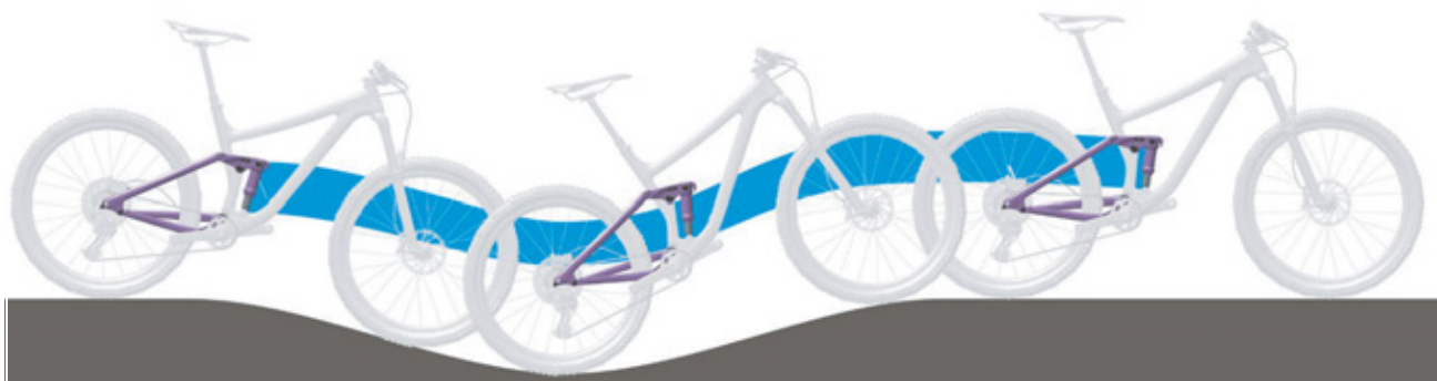
Figure 11: Optimum rear frame damper riding performance on hilly terrain
