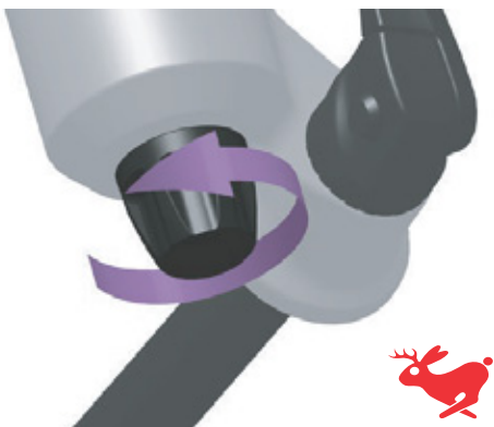
Figure 131: Turning rebound damper towards hare symbol
