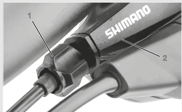
Figure 125: Adjusting sleeve (1) for the single-cable, cable-operated gear shift with shifter housing (2), example
