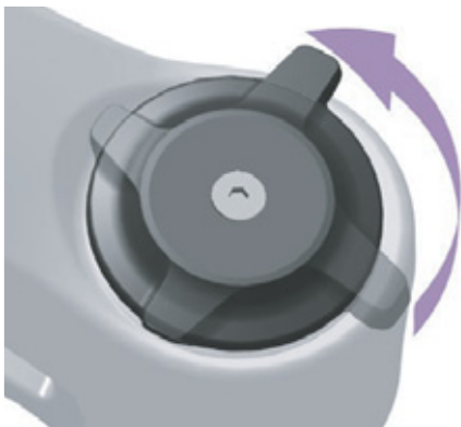
Figure 135: Changing compression adjuster to a softer setting
