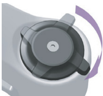
Figure 133: Changing compression adjuster to a harder setting
