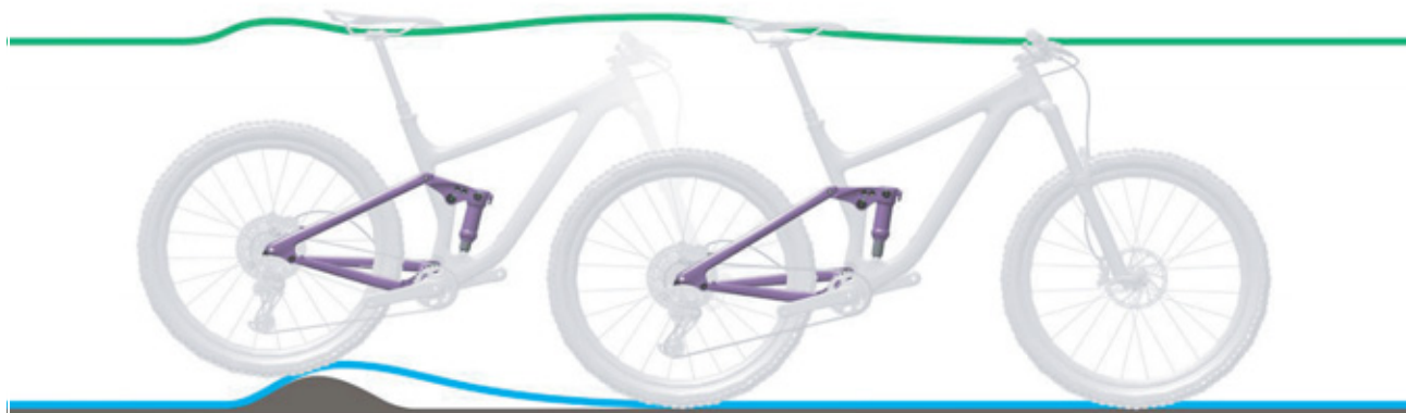
Figure 142: Excessively hard damping in the rear frame damper on bumps
