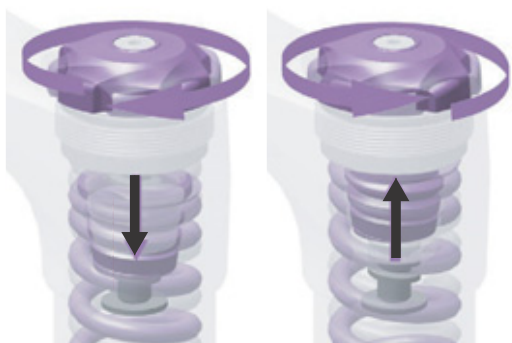
Figure 79: Screwing and unscrewing the pre-tension adjustment ring.
