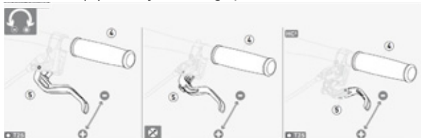
Figure 75: Setting the grip distance on a Magura disc brake lever
