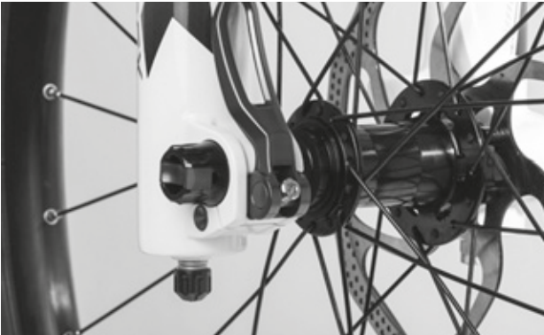
Figure 123: Adjusting the quick release clamping force
